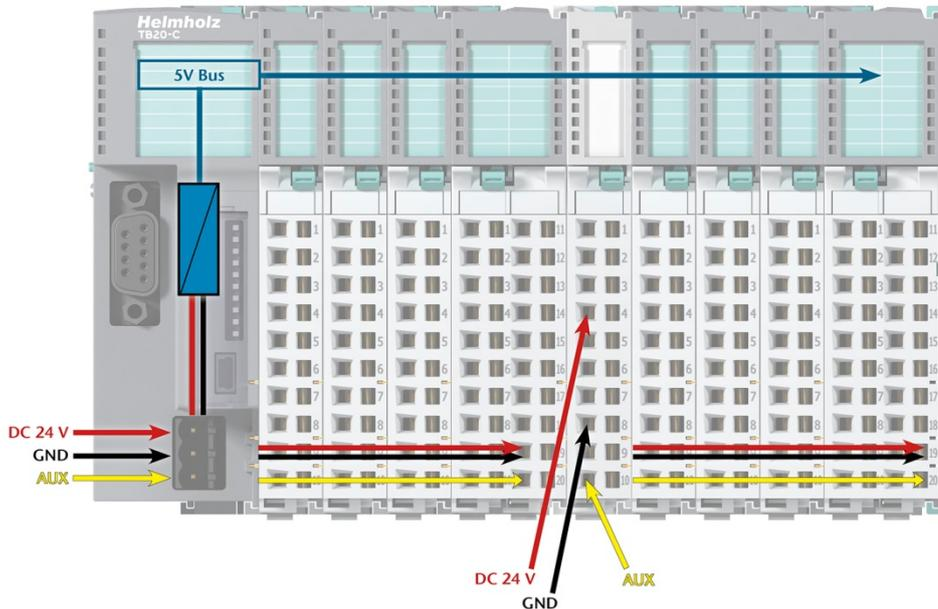
The order No. for the power and isolation module for 24-V signals is 600-710-0AA01.
