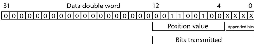
From the bits transmitted, bits 4 to 12 are needed in order to evaluate the encoder position.
