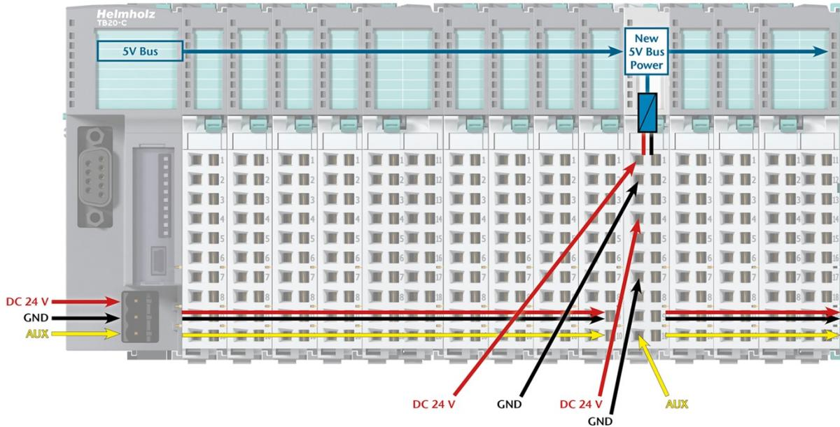
The order No. for the power module is 600-700-0AA01. Its electronic module has the same light gray color as the front connector, while its base module is light gray with a dark core.
