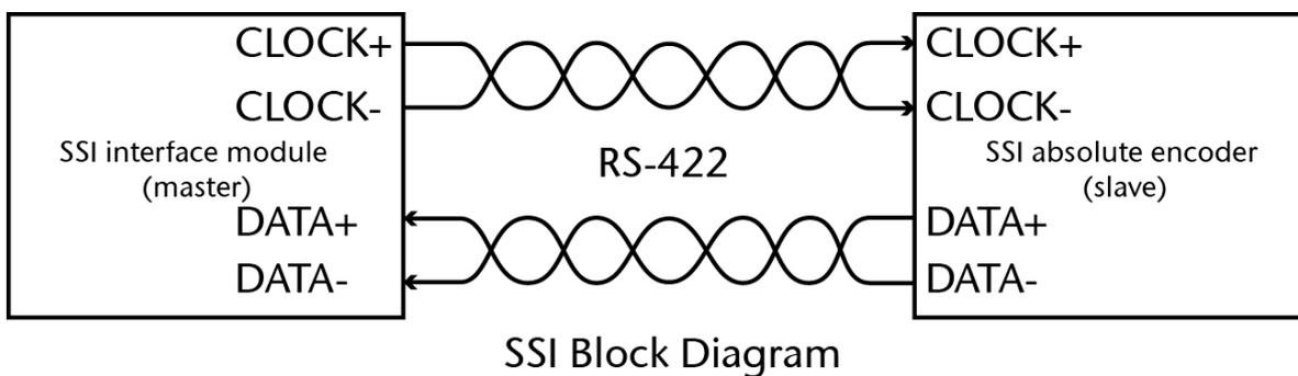
SSI provides several crucial advantages when compared to other interfaces for position measuring systems:
