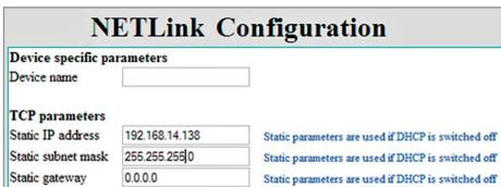
**7. Now, for example, in the configuration screen of the device name, the IP address and the subnet mask of the adapter can be reconfigured and saved in the device. The NETLink® PRO PoE can then be accessed in the network using an IP address changed here.**
