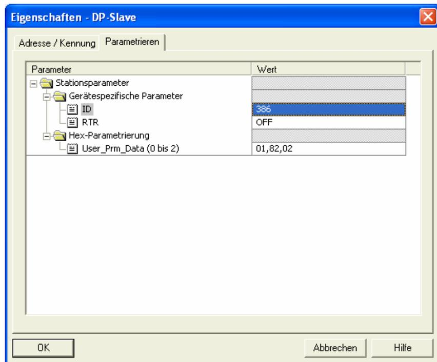
Each transmit or receive object can be defined for exactly one CAN message. The length of the CAN message corresponds to the size of the DI/DO object. The CAN ID is defined in the parameter set.
