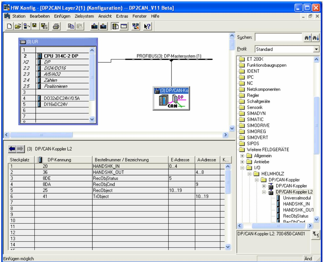
You can assign a station address to the slave here.
