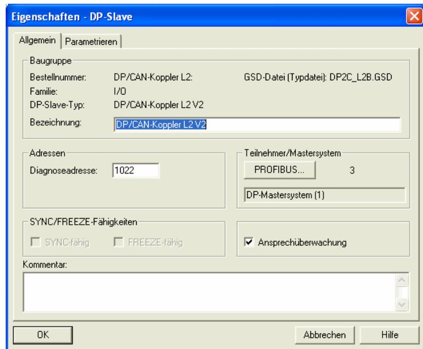
The DP/CAN coupler is supplied with the necessary information with the parameterization frame from the master on start-up about the CAN frames to be processed.
